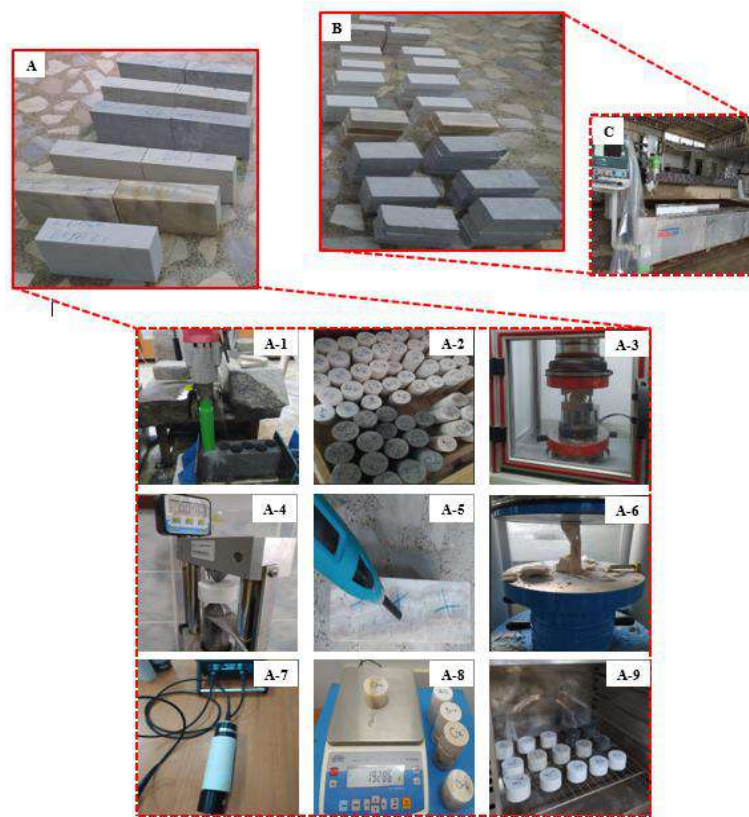
Figure 2. An illustration of the rock samples. A: Block samples for determining the physico-mechanical properties, B: Plate samples for the experimentation, C: AWJ machine used for the experimentation, A-1: Coring process, A-2: Core samples, A-3: Brazilian tensile strength test, A-4: Point load strength test, A-5: Schmidt Hammer hardness test, A-6: Uniaxial compressive strength test, A-7: Ultrasonic velocity test, A-8 and A-9: Water content test
