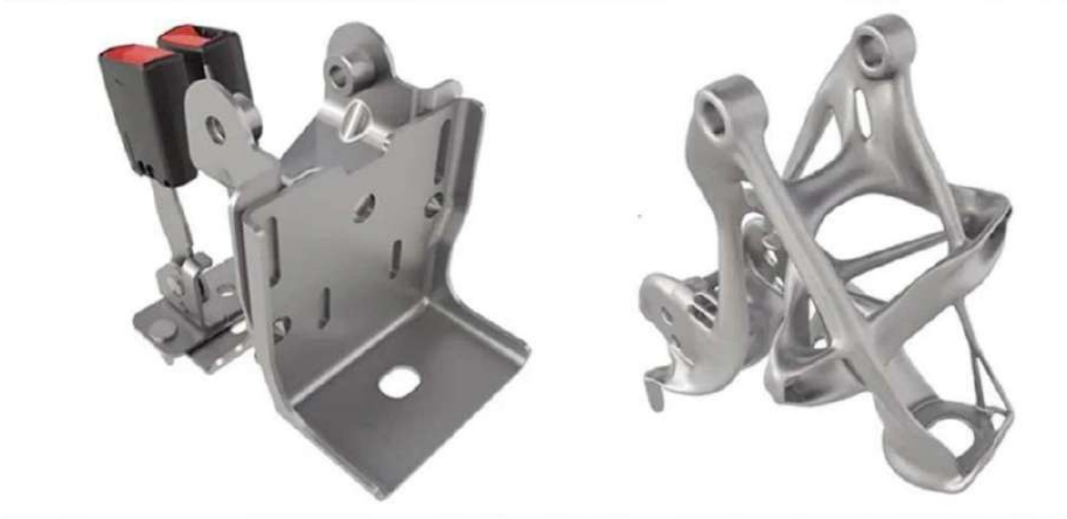
Figure 5. Utilizing additive manufacturing in the production of parts, General Motor Thanks to 3D printing, he succeeded in creating the piece, which was created by combining 8 different parts, in one go. (Courtesy of General Motor).
