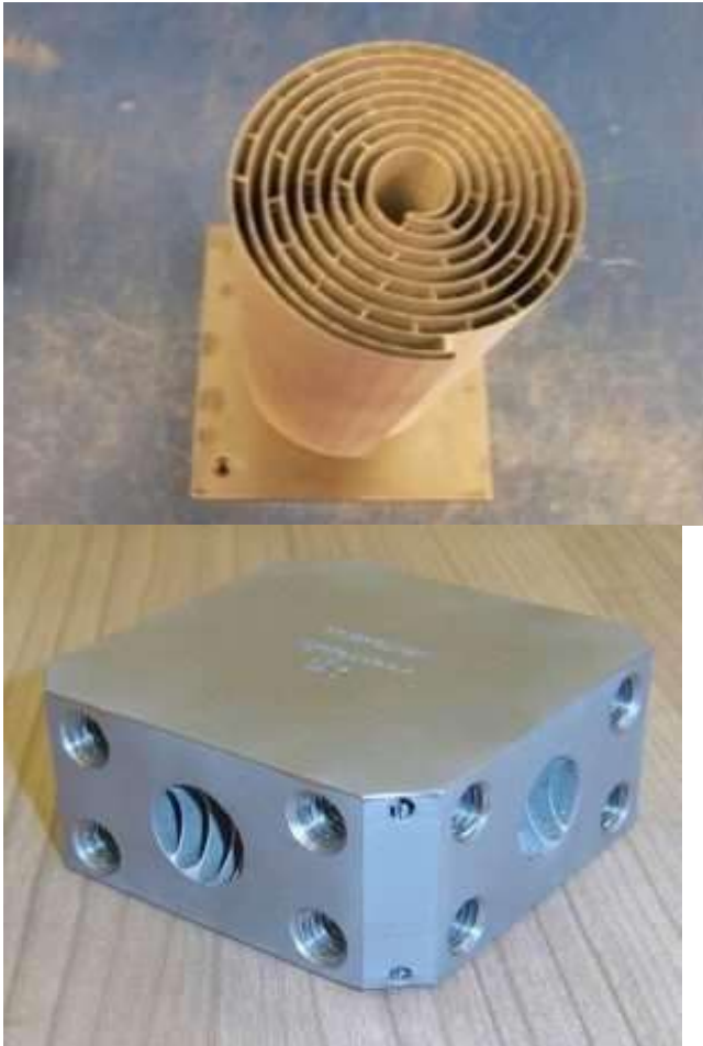
Figure 4. Hydraulic prototype with complex internal channels, (Source: EU project COMPOLIGHT) (Left). (b) Prototype of 316L vacuum permeator for ITER, produced by LBM, impossible to manufacture by conventional processes. (Courtesy of IK4-Lortek) (right)
