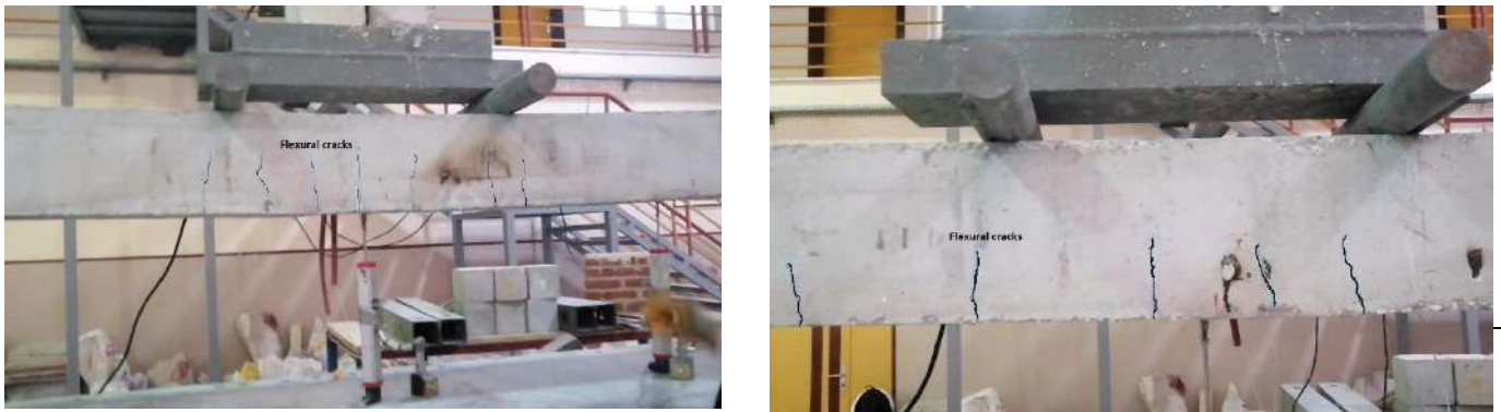
a b Figure 9. Typical flexural cracks in test elements (a) S1 (b) S2
