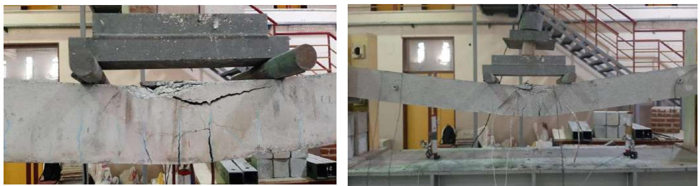
a b Figure 9. Typical flexural cracks in test elements (a) S1 (b) S2
